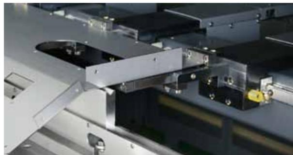
Materials can be placed on the upper surface of the Finger support part, therefore, stable processing is enabled without material crowning in the case where a deep material is bent.
