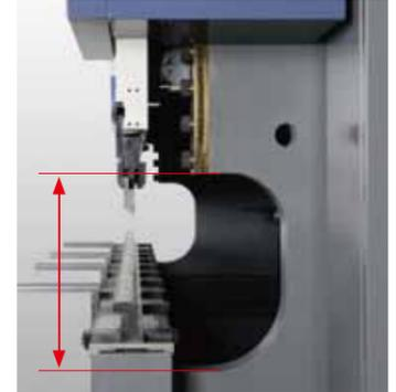
The open height (100 mm wider than standard) specification is set optionally. This improves work handling performance for the deep bending process which is frequently used for processing control panels.
