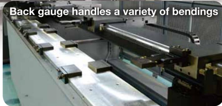
The high-speed and high accuracy back gauge with an effective stroke of 700mm (standard specification) responds to a variety of bendings. Number of fingers: 2 (Option 4)
