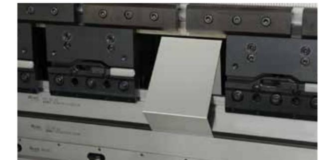
The intermediate plate of the tool clamp can be freely removed, therefore, bending processing which interferes with the deep U-shaped ram is enabled depending on the size.
