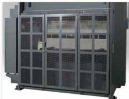
Intrusion to movable parts from the rear part of the machine is guarded to prevent unexpected hazards and ensure safe work. When the rear safety fence is opened, the machine is inoperable until the interlock is released.
