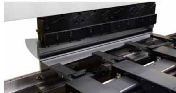
The back gauge can be tilted obliquely, it is thereby possible to easily perform obliquely abutting, etc. Depending on the shape, conical bending processing, etc., is enabled.
