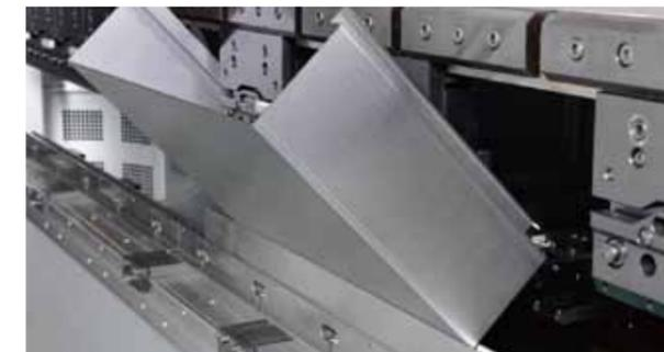
The height of the intermediate plate of the tool clamp is 150mm to allow for freely moving in the right and left directions, therefore, deep bending (box bending) processing which is common for distribution boards is enabled.
