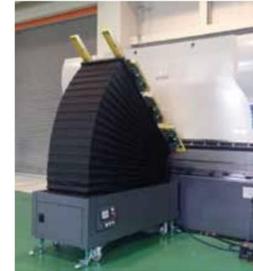
Useful for bending large-sized and heavy workpieces and considerably reduces burden on operators. The weight capacity is 150 kg. Two suction types, a magnet type and a vacuum type, are available.
