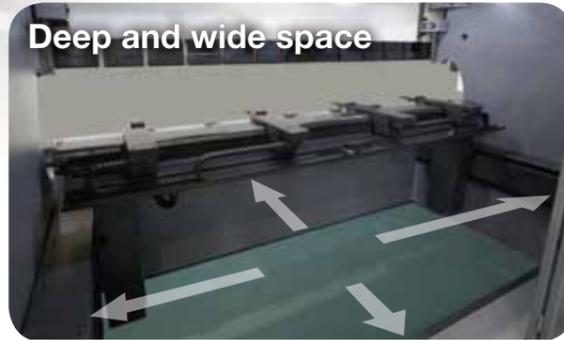
The back gauge main body is placed on the side frame to secure a deep and wide space. This enables handling a wide variety of workpieces.
