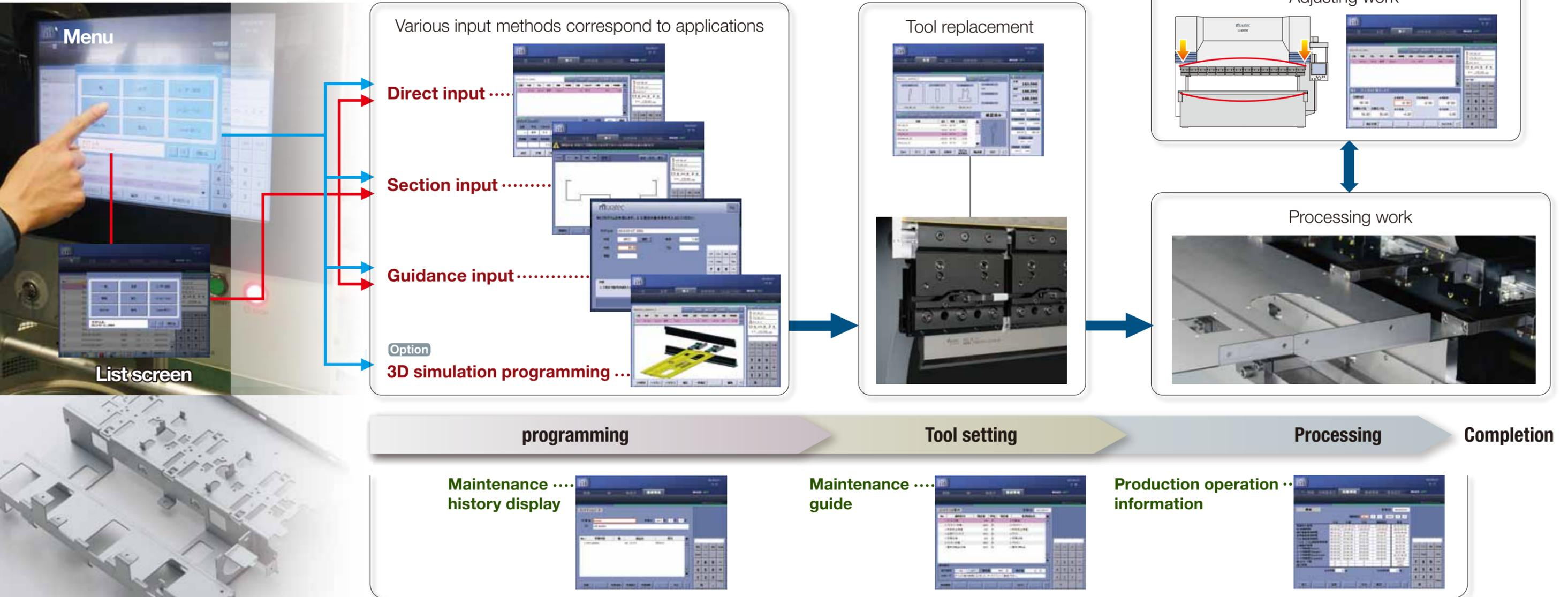
The control system with a panel computer mounting 2.2GHz Dual-Core processor and 15in TFT touch panel is a user-friendly control system superior in operability.
